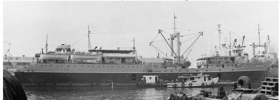
DONA TON after conversion to a cargo vessel, Manila North Harbor 16 June 1970. Awning decks can still be seen behind the bridge (without boat) and forward of the two aft boats (W. Schell)
