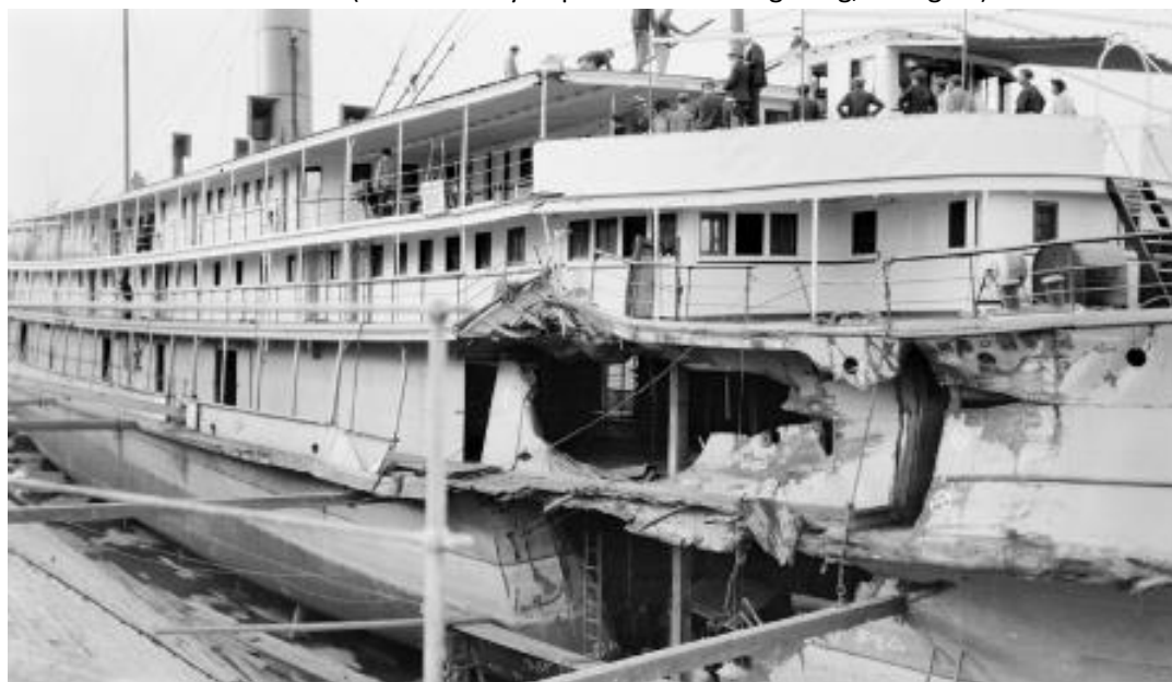
KIANG HSIN being surveyed by dockyard and insurance staff after sustaining damage in an undated collision with YOH YANG MARU. Funnel top and base have been repainted yellow, presumably to safeguard the corporate image (Warren Swire colln).
