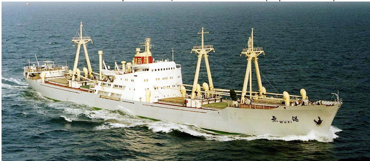
WUXI in the English Channel, fourteen 5-ton and one 30-ton derricks (FotoFlite/coll. Roger Hurcombe permission Nigel Scutt).
