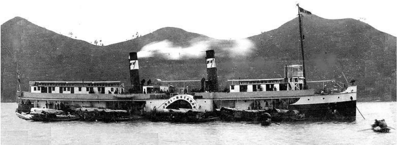
SUI HSIANG at Ichang, mast, lookout, awning frameworks fitted (University of Toronto/SK edit).
