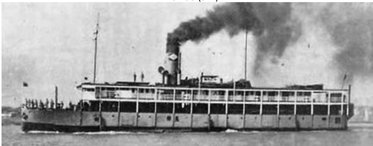
MING HSU with flush main deck and mainmast post-1948 ( Shanghai 100 year shipbuilding history ).
