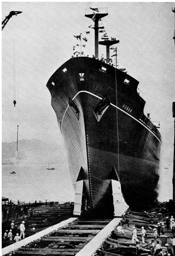
HUNAN's launch, 25 Oct. 1965, showing her fine lines (no bulbous bow) ('Taikoo Dockyard', No. 20/1966).
