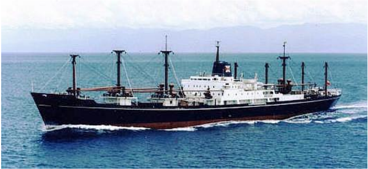
HUNAN in St George's Channel at speed with 'a bone in her teeth'. By 1968 new ships would have bulbous bows to smooth the bow wave and reduce friction (CNCo).
