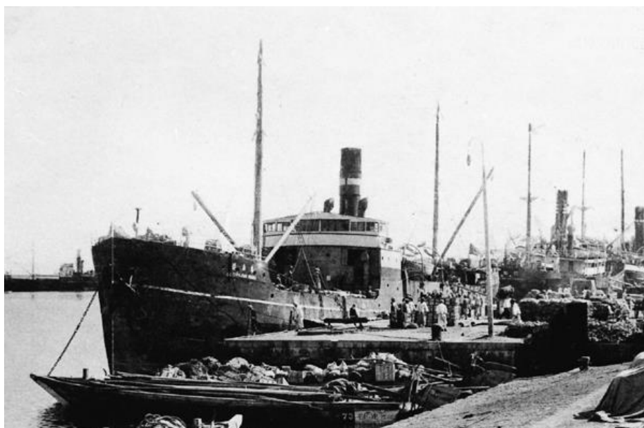
SAKURAJIMA MARU in Chosen Yusen colours. High superstructure side plating was a characteristic of 1920s Harada-built steamers (from a postcard).
