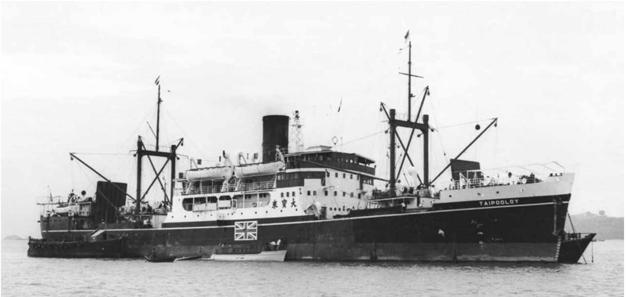
WING SANG (1938-58) as TAIPOOLOY at Singapore c.1960 under Shun Cheung ownership. Main outward change is radar/signal mast on bridge (R. Gabriel*).
