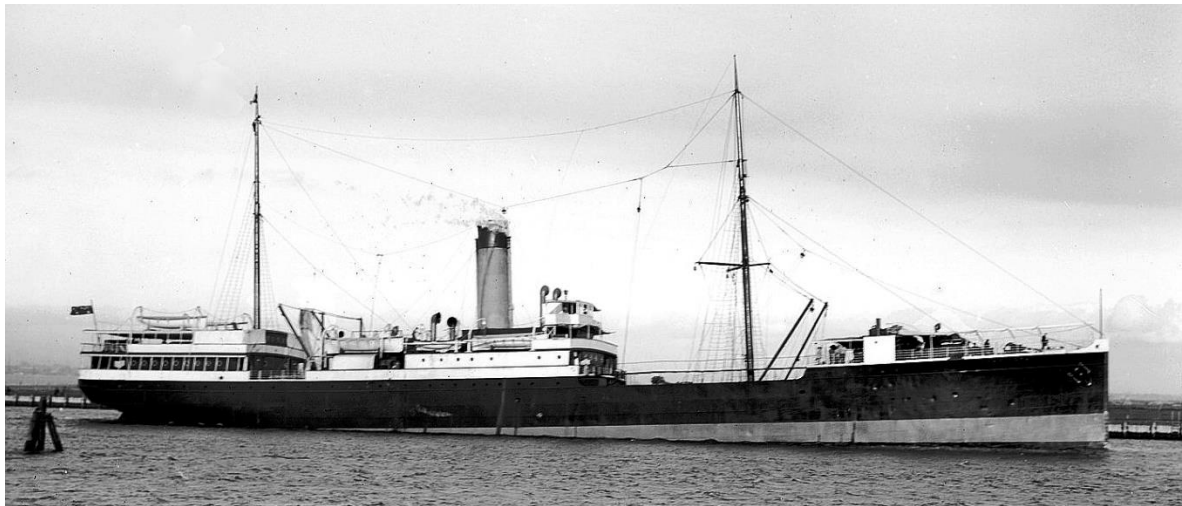
SEISTAN as Adelaide S.S. Co. INNAMINCKA post 1910 with wireless, sails removed (A.C. Green/SLV).
