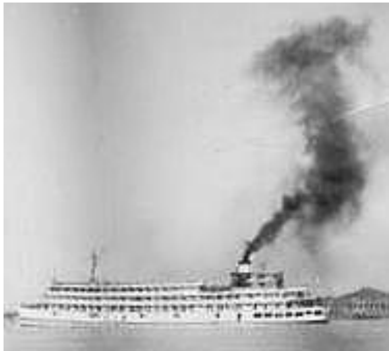
DONG FANG HONG 9. Hatches, cargo gear removed, top deck built up, funnel raised one deck (7788.com).
