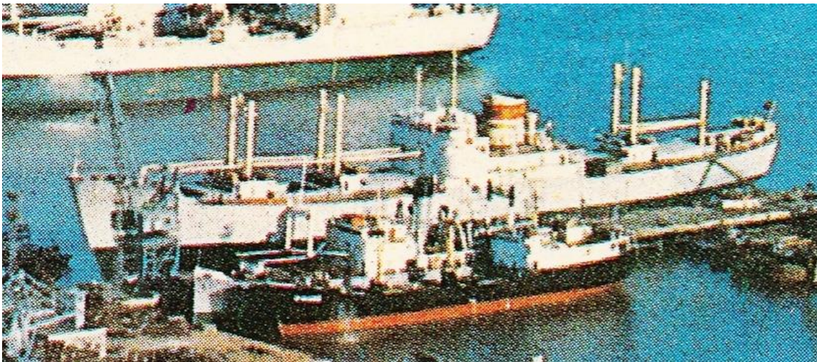
Centre vessel (tall funnel) presumed GONG NONG BING 8 at Tianjin Xingang shipyard from a postcard view 1971 or later. The large COSCO cargo ship is HUANG SHI ex LA ORILLA, the small one with black hull is QIAN SHAO 2 or QIAN SHAO 3 of SMB, managed from Dalian, hull dimensions 230.25' (o.a.), 214.24' (b.p.) x 32.8' (coll. Graham Thompson).
