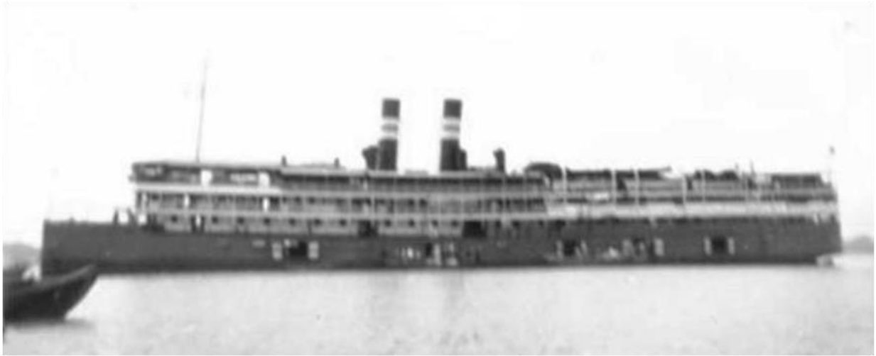
NINGSHIN, reconstructed with full new upper deck (Virtual Shanghai).
