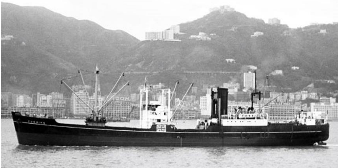
FUCHING at Hong Kong, 31 May 1964. Samsons on fo'c'sle and poop have been removed and prominent Union Jack on plated up bridge deck (Dr. George Wilson).
