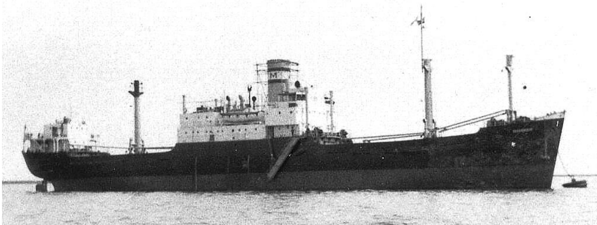
TEES BREEZE with scaffold around a bigger funnel replacing the original stovepipe (SK*)
