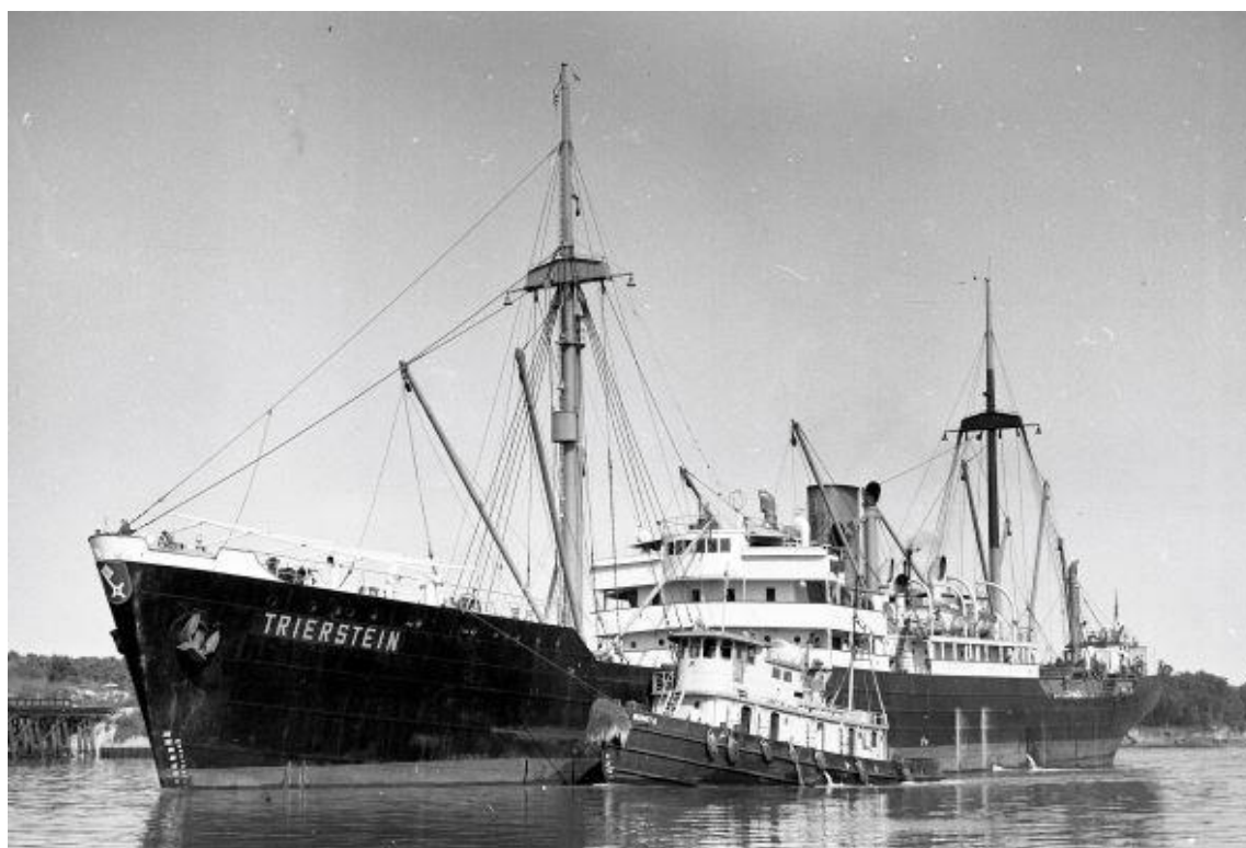
AMONEA (III) as NDL's TRIERSTEIN in Houston Ship Canal, May 1955, with longer, streamlined bow section (1939) (P. Myers/W. Schell).
