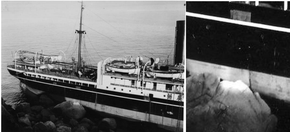
KWANGCHOW on rocks showing hull fracture leading to CTL (coll. SK).
