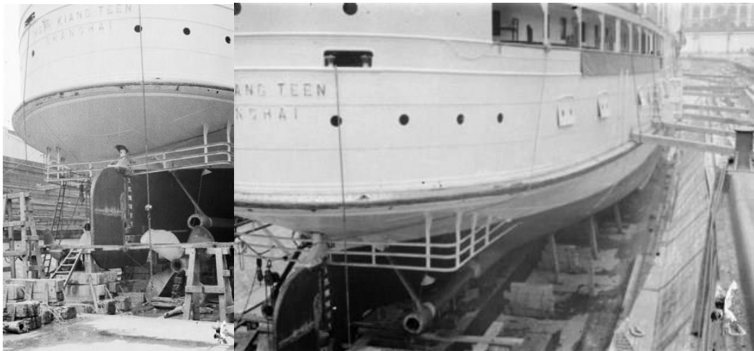
Damaged propeller blades under repair, Shanghai 1937 (Harrison Forman, UWM Libraries).
