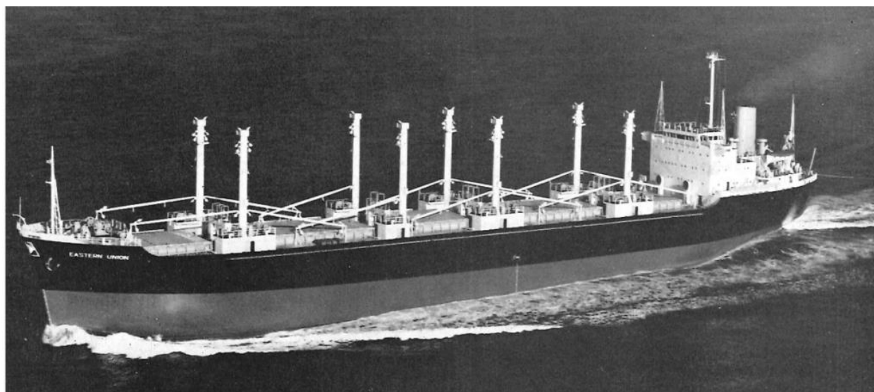
EASTERN UNION working up 16.72 knots on trials ( Fune no Kagaku 3/67).
