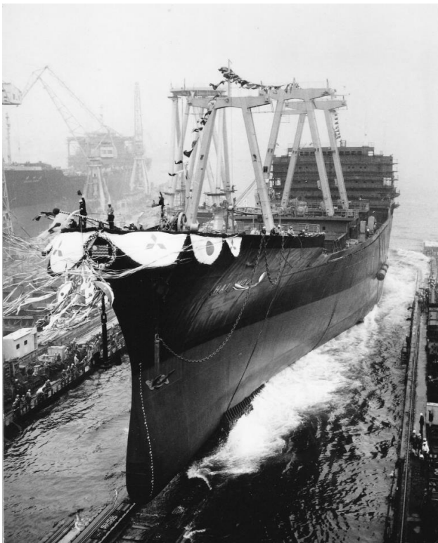
Launch of HAI MOU, showing bulbous bow (builders*).
