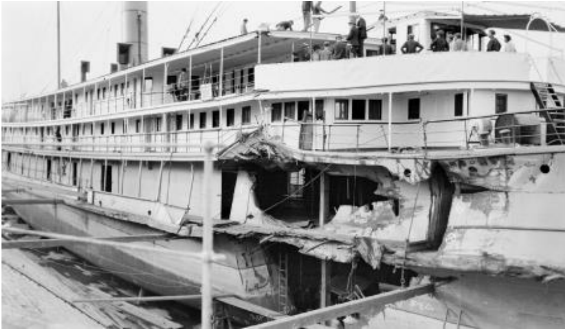
KIANG HSIN being surveyed by dockyard and insurance staff after sustaining damage in an undated collision with YOH YANG MARU. Funnel top and base have been repainted yellow, presumably to safeguard the corporate image (Warren Swire colln).
