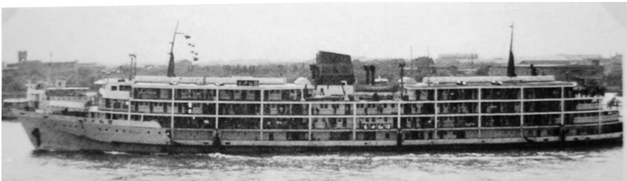
DONG FANG HONG 10. Forward section rebuilt similar to DONG FANG HONG 1 and DONG FANG HONG 7. Aft two-thirds very similar to DONG FANG HONG 4 (Furukawa).
