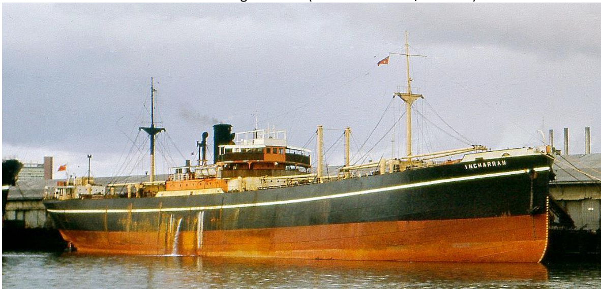
INCHARRAN at 5 Glebe Island, Sydney, 29 June 1963 to load wheat for Persian Gulf. Prominent stovepipe added above the poop as exhaust for the Chinese crew's galley (A. Travers/NAA).
