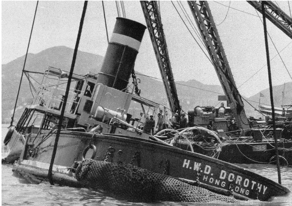
HWD DOROTHY being raised, 7 Sept. 1962, gashed amidships (The Standard, 8/9/62).
