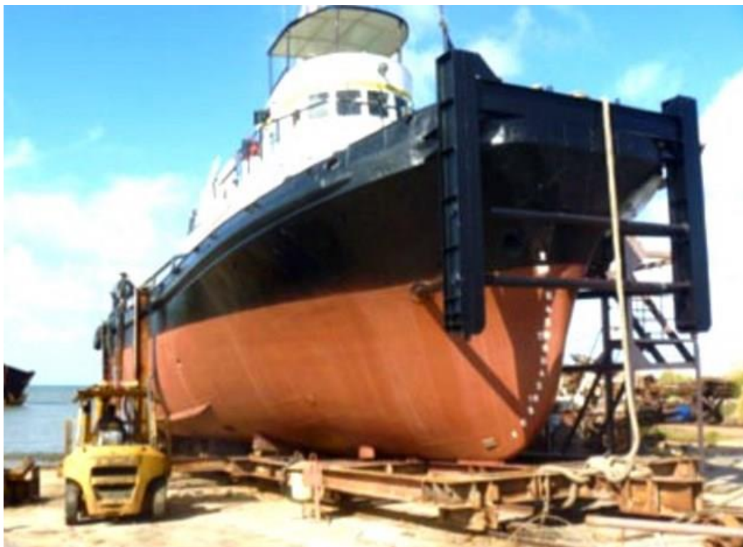
Ex LAIMUN/ BANDURRIA I under conversion to pusher tug ( marinamercanteuruguay.blogspot.com ).
