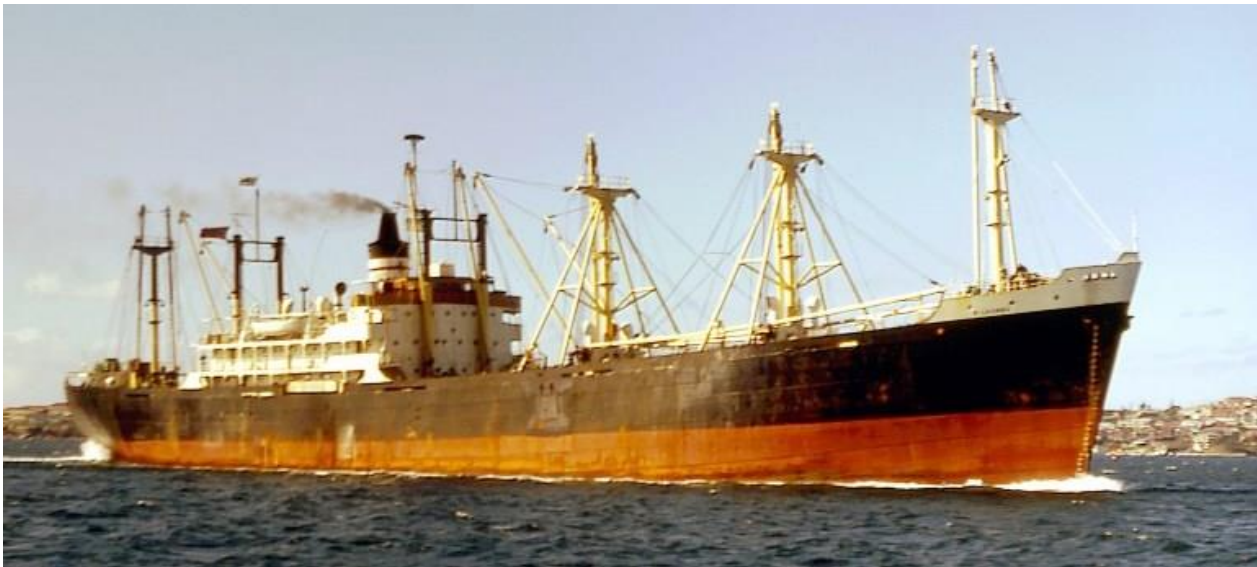
BILKURRA at Sydney after masts stiffened for lifting containers (Reg Wilson).
