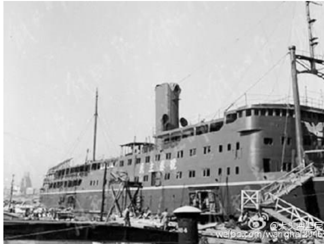
MIN CHU 3 with a new superstructure front, under refit at Shanghai (weibo.com).
