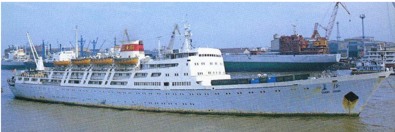
CHANG ZHENG's forward cranes were subsequently replaced by containers
