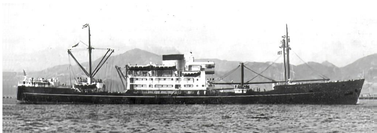
EASTERN QUEEN as originally built for the Calcutta line with squat funnel and minimal plating around the centre island (JM&C).
