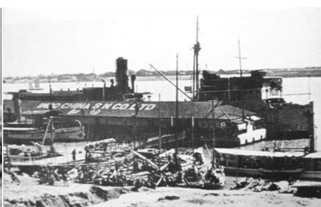
PING WO at Ichang in 1926, and in the late-1930s on the outside berth at Hankow. Superstructure now closed in forward and extended aft, but still good facilities for cargo-carrying (L: John Swire & Sons, R: China Proper Vol III ).
