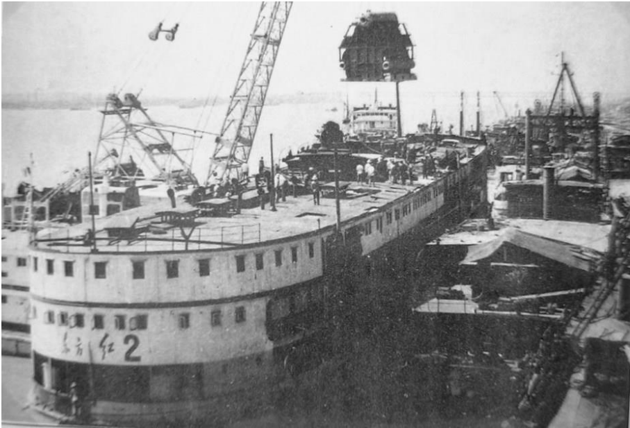
DONG FANG HONG 2 ex-YOH YANG MARU under major refit in 1966, evidently receiving a new main boiler ( The Yangtze River ).
