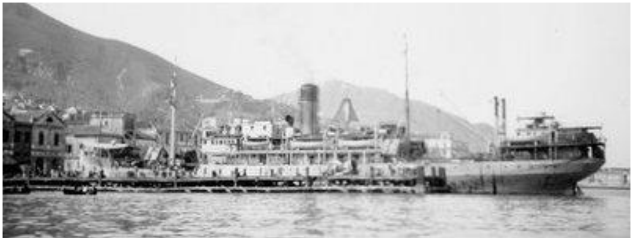
YUEN SANG in 1945/46 with superstructure enclosed forward (NMM).
