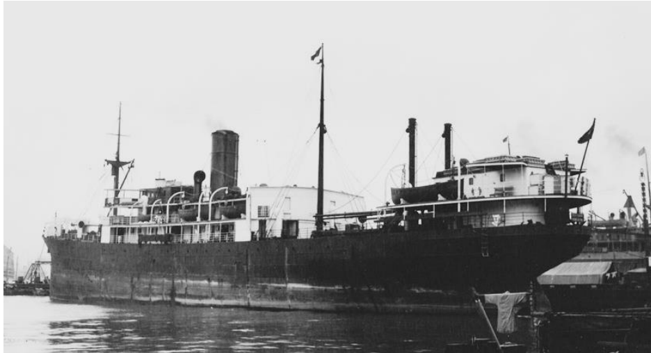
Kowloon, 7 April 1940 showing prominent anti-piracy barricade, forward well evidently eliminated (D. Gammon*).
