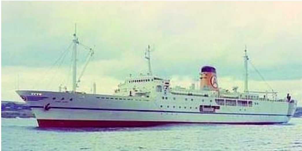
KOBE MARU was built to operate a fast (22.5k) connection between Okinawa and Honshu ( https://img01.ti-da.net/usr/minokasigo/ ).
