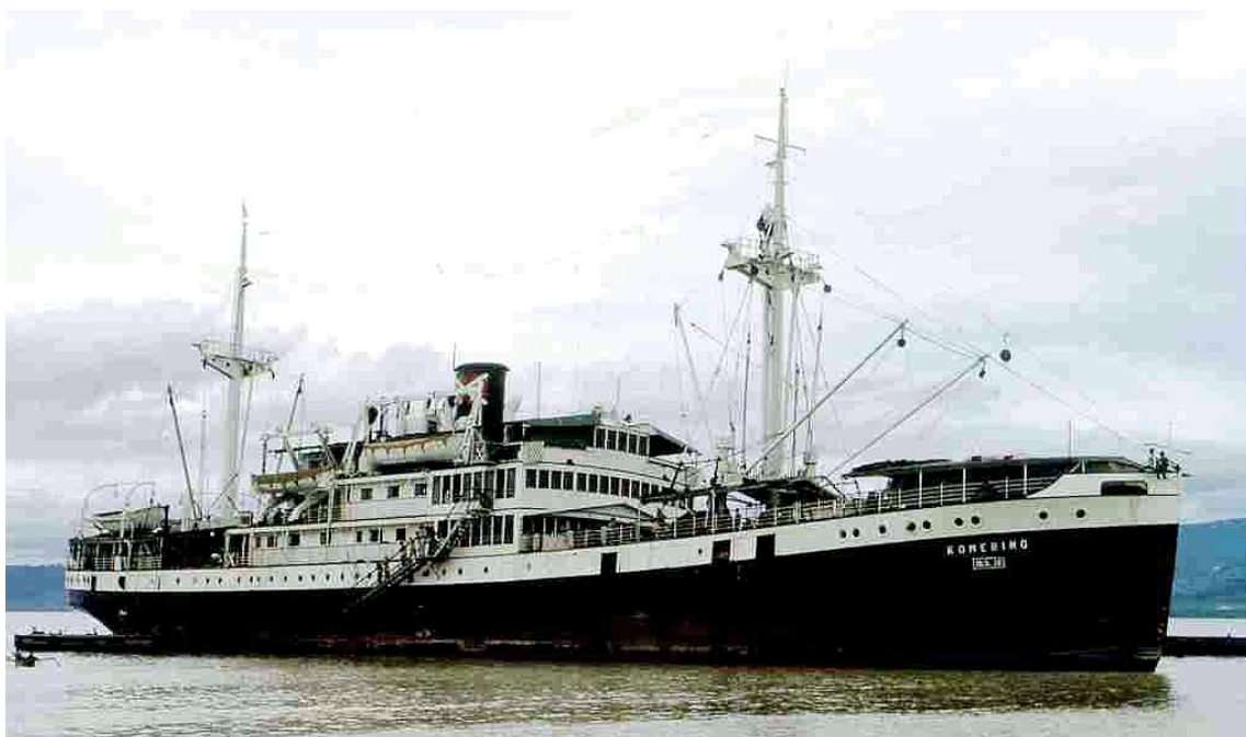
KOMERING at Donggala, late January 1974, large windows in forward superstructure, some sideports open, awnings removed over hatches (H. Dick).
