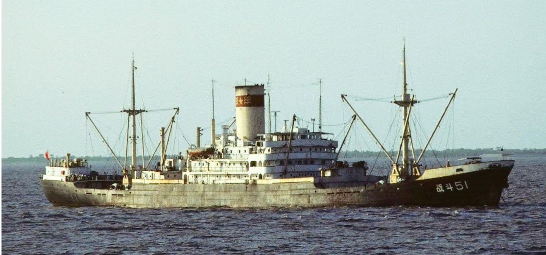
ZHANDOU 51 ex HONG QI 119 in Yangtse delta, three pairs of kingposts removed (Donald Anderson).
