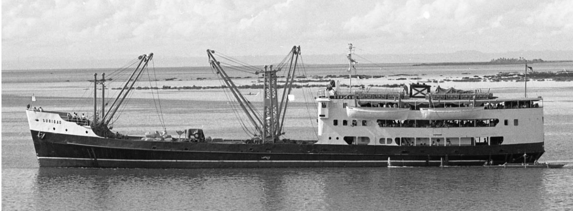
SURIGAO, Cebu 9 June 1970, updated with extra deck and extra hatch (W. Schell).
