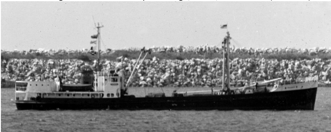
ROSARIO in 1971-75 at Guam, new derricks, stern enclosure for extra cabin area (Bob Tomkins).
