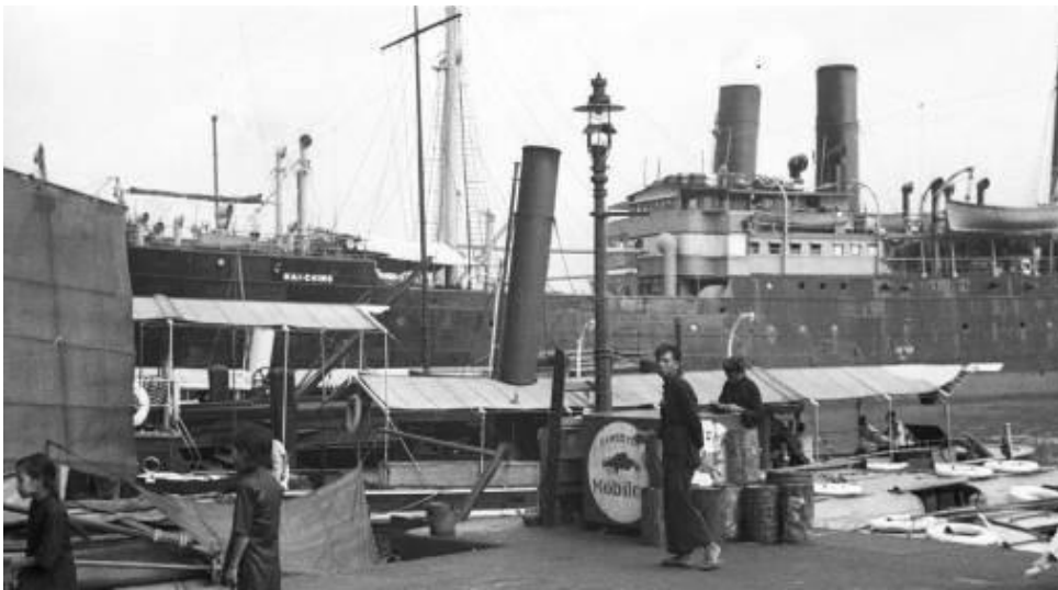
HAICHING at Hong Kong, probably on 16/9/40, after further reconstruction with more enclosed superstructure, upright masts and funnel, and kingposts on fo'c'sle. SEISTAN behind and small DSSC tender in foreground (Harrison Forman/University of Wisconsin-Milwaukee Libraries).
