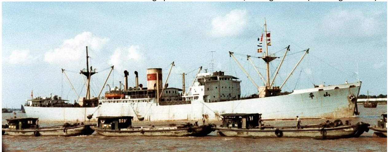
HUA SHAN at Shanghai 20 July 1979, additions to front and centre superstructures (Markus Berger).
