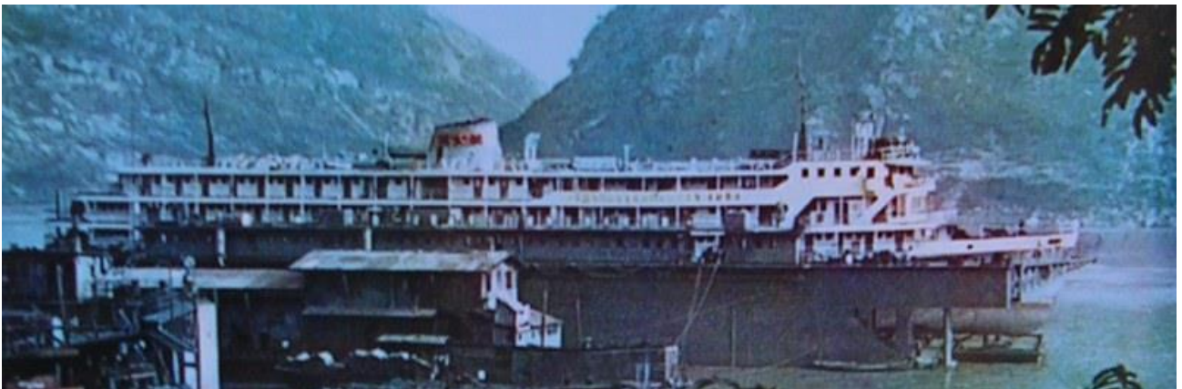
Lengthened DONG FAN HONG 31, extended upper deck
