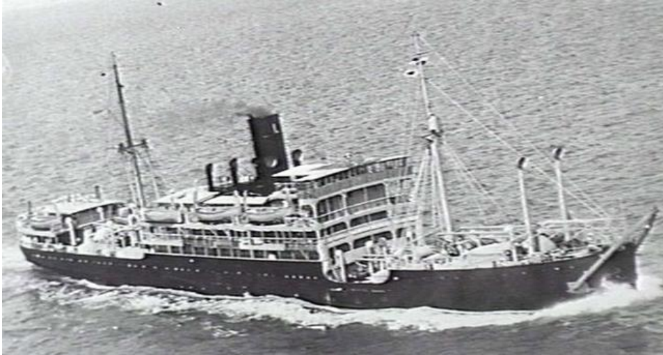
TAIPING on 21 Dec. 1940 with a frame for paravane gear fitted at the bow (AWM303999)
