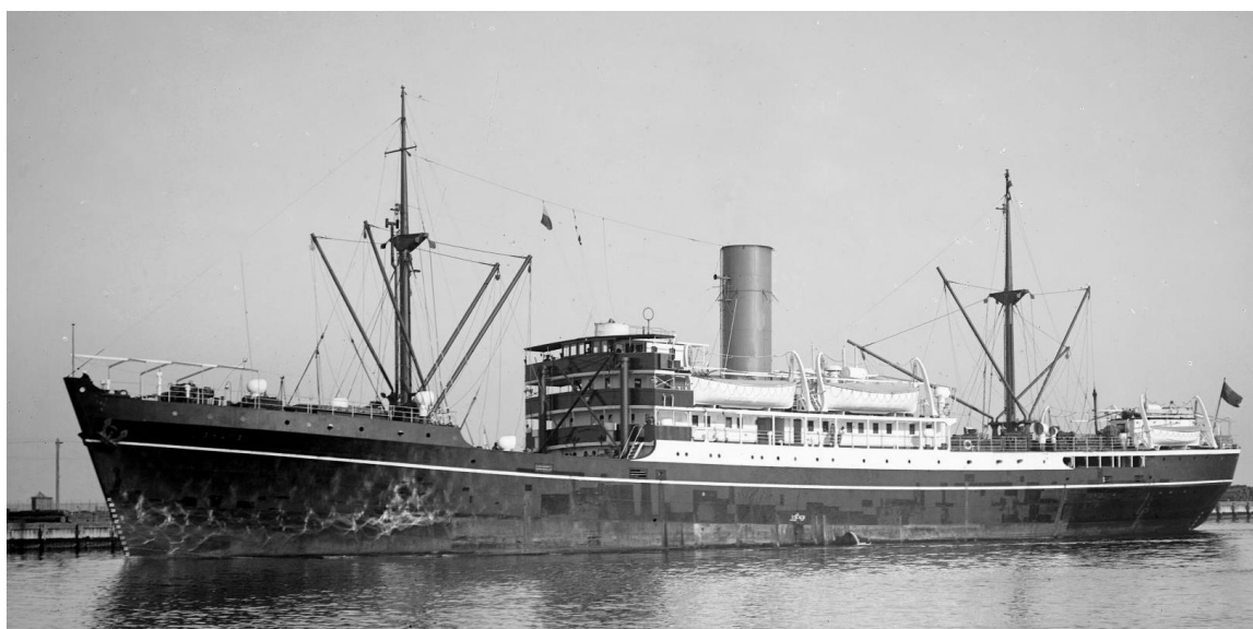
SHANSI arriving Melbourne with buff funnel while on Australian Oriental Line charter, still with open plating in way of No. 4 hatch, long forecastle and bow knuckle clearly seen (A.C. Greene/SLV).
