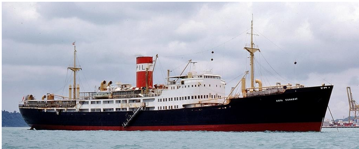
KOTA SAHABAT looking smart at Singapore on 1 March 1978. Livestock pens on the after hatches and poop and even on the Boat Deck. The tall ventilators are new additions, as are the similarly buff-painted, square fodder lifts (Chris Gee).
