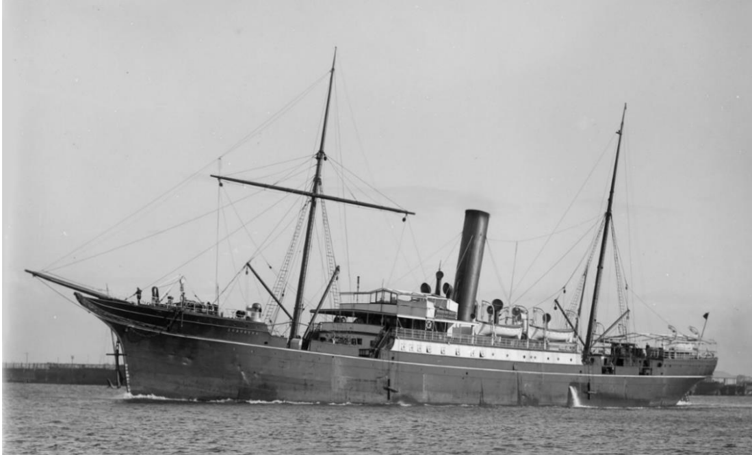
CHANGSHA of 1886, sold to AOL in 1912. Here reduced from original rig. The crossed yard was later removed (A.C. Green/SLV).
