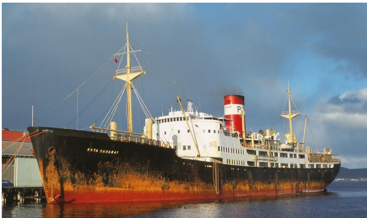
KOTA SAHABAT at Hobart on her second last voyage, 17 September 1979, the hull but not the upper works showing obvious signs of neglect (R. Cox)
