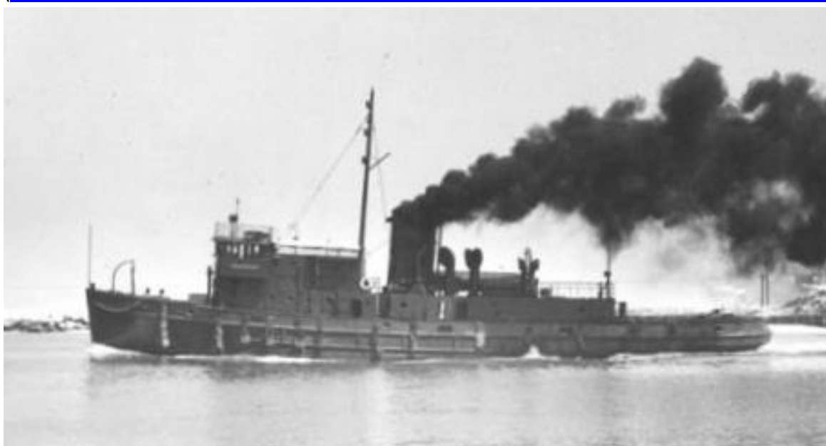
'Type 254' tugs had a 3cy uniflow steam engine. Image shows ex-LT-651 ( http://eshore.iath.virginia.edu/node/5965 ).
