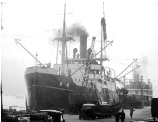
Left: LAKE STRYMON (Bowling Green State University). Right: QIN JIAN, unidentified former 'Laker' at Shanghai 20 December 1963. Evidently re-equipped with new masts and heavy cross-trees (SK*).
