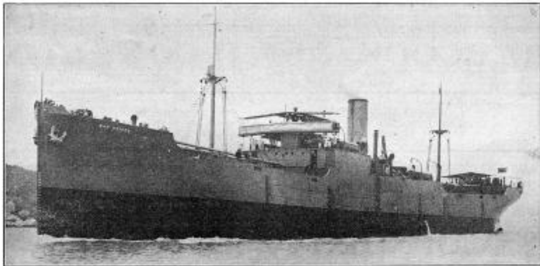
H.B. "WAR SNIPER," 8,200 tons d.w.,—3,175 tons gross. Built and engined by The Hongkong & Whampoa Dock Co., Ltd. to the order of the British Government.
