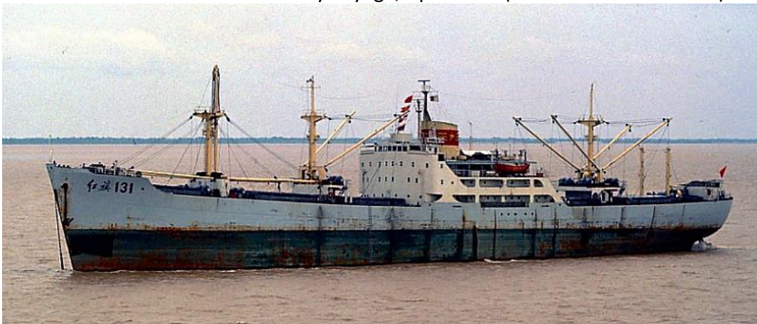
HONG QI 131 at Shanghai, 1982-3 (Chris Mackey). Deck beneath bridge now fully enclosed.
