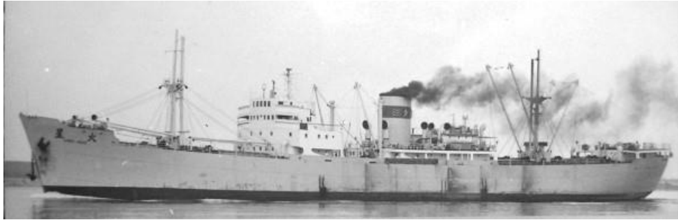
XING HUO later HONG QI 130 at Rotterdam, 21 June 1970. Superstructure front enclosed for extra accommodation (Malcolm Cranfield).
