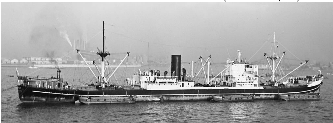
INCHMAY at Nagoya, 24 November 1964, extra accommodation abaft the bridge and on boat deck, twin stovepipes at poop for the Chinese crew's galleys (Dr. George Wilson)
