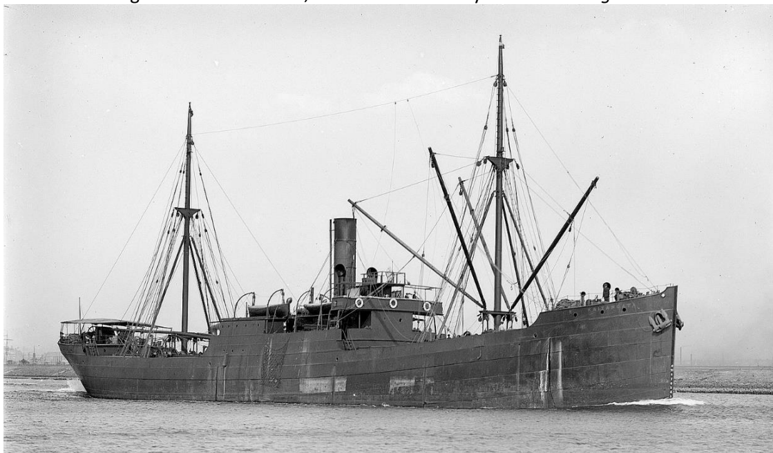
Union Co. KAITANGATA in the Yarra River with coaling gaffs raised at foremast (A.C. Green/SLV).
