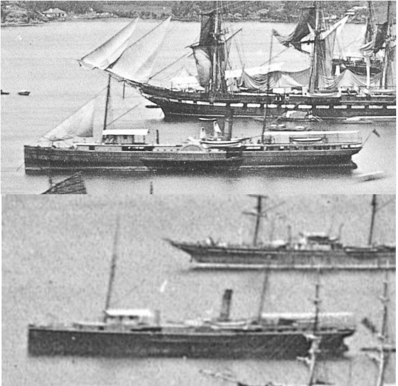
Above 2 photos: NANZING at Nagasaki minus a funnel in 11/74 to 2/75. First photo also shows missing top mast and torn mainsail (Nagasaki Univ 5301, 5299)
