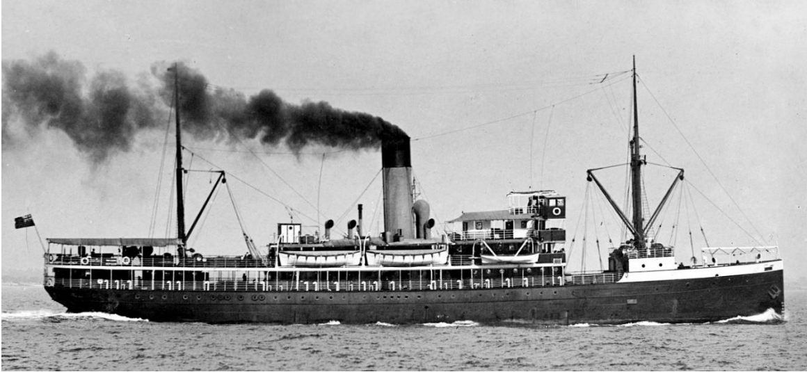
Adelaide S.S. Co. MORIALTA dep. Melbourne while in Queensland service. As built with low fo'c'sle and flying bridge plus radio aerials (A.C. Green/State Library of Victoria).
