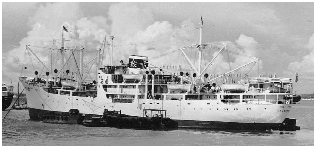
Above 2: HOI YING with Ngow Hock funnel, 'tween deck with portholes, 10 ventilators, 8 boats plus rafts (P. Foxley; unknown photographer/coll. S. Kentwell).
