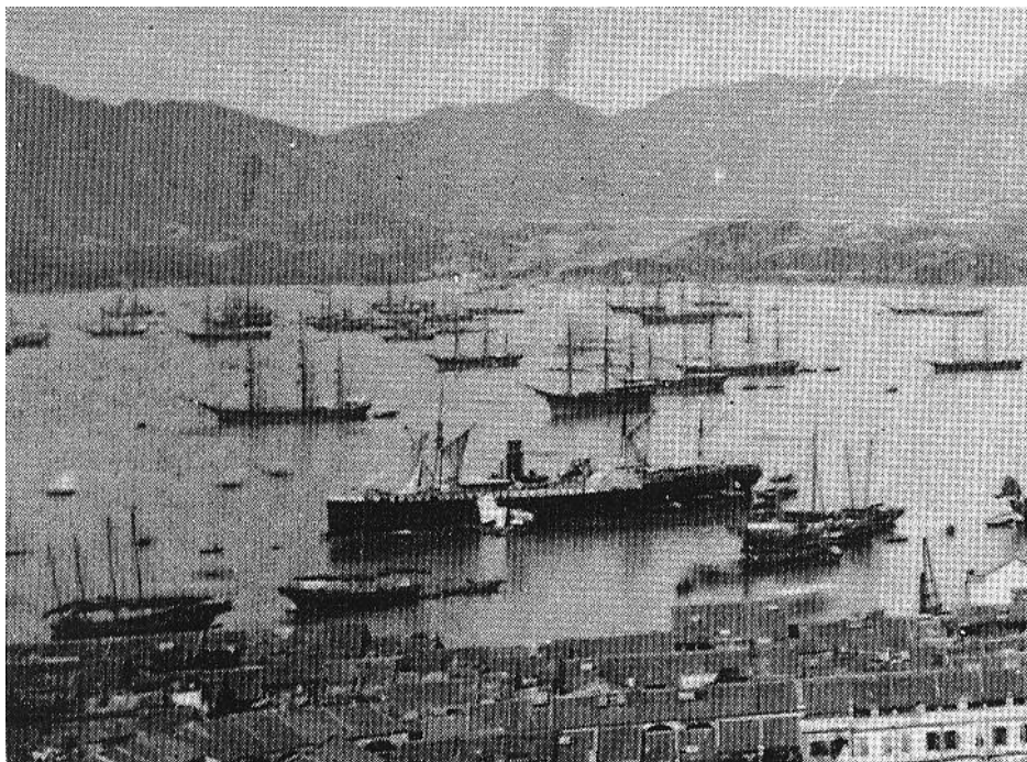
One of the four sisters at Hong Kong, fewer cross-yards, superstructure layout and paddle box design suggest this might be the AMERICA (HKMOH).
