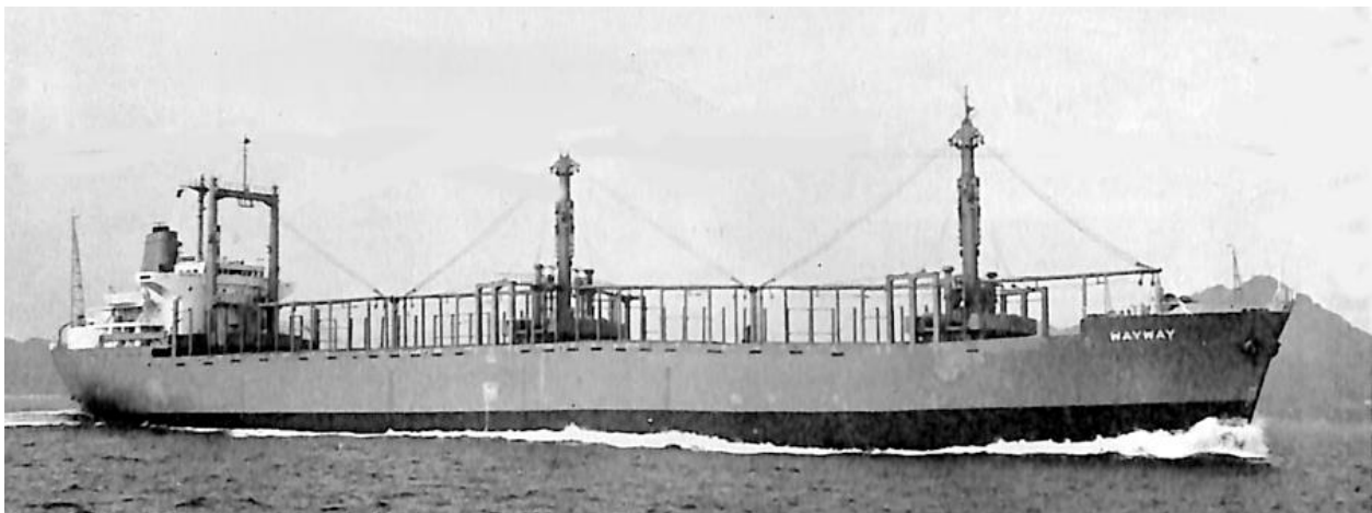
WAYWAY on trials with stanchions for on-deck logs (Hitachi Zosen).
