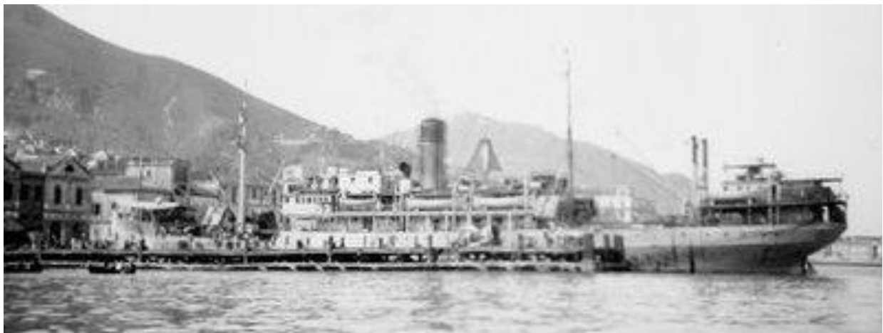
YUEN SANG in 1945/46, top deck enclosed forward but not fitted with anti-piracy plating (NMM).
