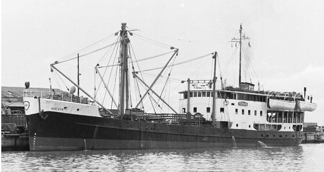
Converted and lengthened FS-405/VIZCAYA under Philippine S.N. Co. ownership at Manila North Harbor, 11 June 1970, kingposts against bridge (W. Schell)
