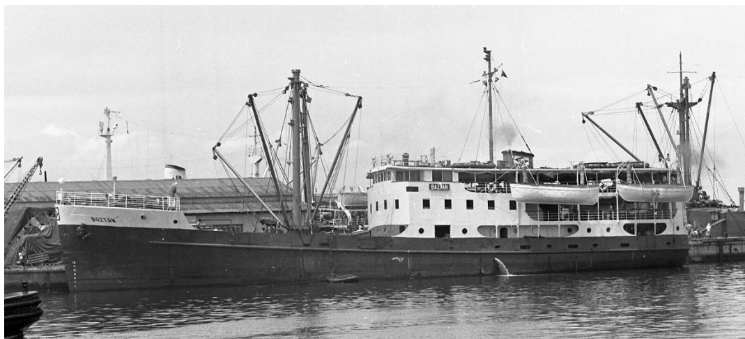
Converted BAZTAN at North Harbour, Manila on 16 June 1970 in Philippine S.N. Co. colours. Heavy lift at No. 2 hatch and three accommodation decks (W. Schell).
