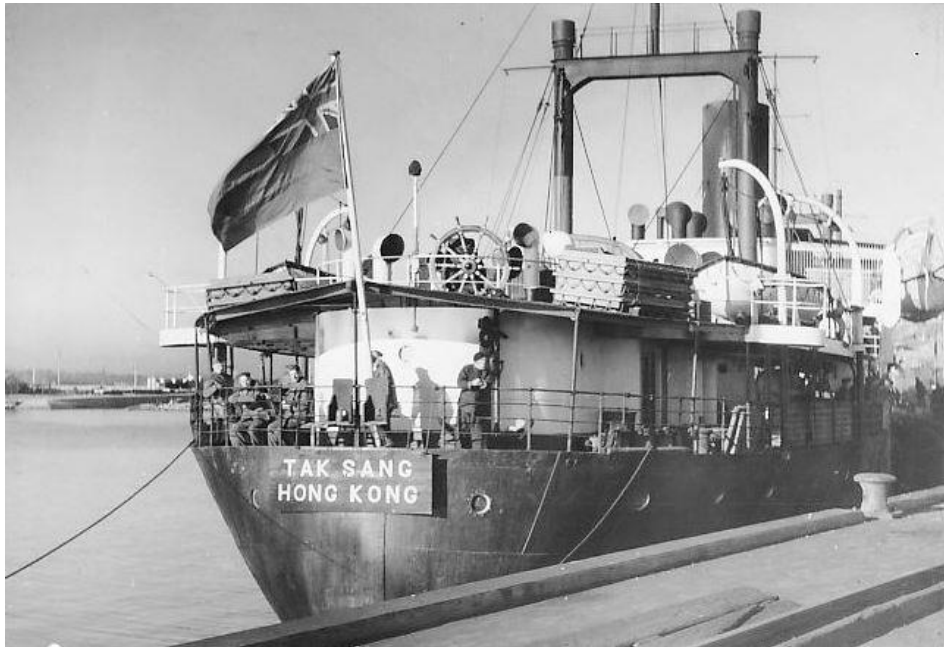
TAK SANG with removable nameboard, evidently re-shortened funnel, presence of military personnel, and absence of hull band in an unsourced photograph dated 12 March 1939.
