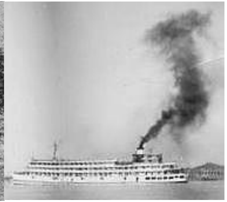
Left: PAOWO at Hankow, prewar. Hatch abaft bridge as per KUNG WO and PING WO (SK). Right: DONG FANG HONG 9. Hatch removed, top deck built up, funnel raised one deck (7788.com).
