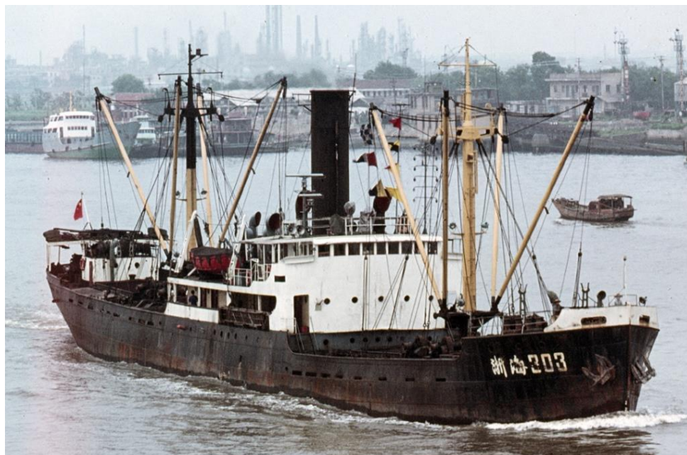
Above 2: ZHE HAI 303 ex AGUADULCE arriving Shanghai on 18 June 1982 with new masts, superstructure plating, hull openings and portholes (Chris Mackie).
