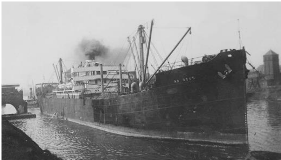
ABERCOS photographed in the Manchester Ship Canal with topmasts struck to pass the bridges (from a postcard).
